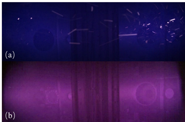
FIG. 8. Plasma discharge images for different vacuum environments: (a) Shot No. 210523021: the vacuum environment is bad; and (b) Shot No. 220914026: the vacuum environment is good.
